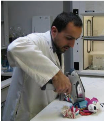
Trace personnel performing XRF Testing of Children's Product
